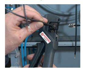
Professional contact crimping tool with interchangeable dies for the installer or service technician.
