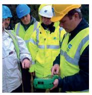
Measuring earthing resistance of the earth connection
