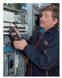
Elpress Mobile, professional tool with interchangeable dies for the installer or service technician.
