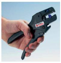
EMBLA, ergonomically adapted cutting and stripping tool.
